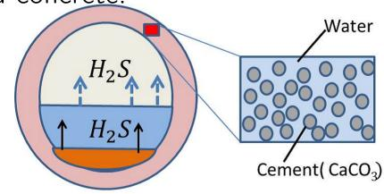
$$\begin{aligned} & \text{H}_2\text{SO}_4 \rightarrow 2\text{H}^+ + \text{SO}_4^{-2}, \\ & 2\text{H}_2\text{O} + \text{H}^+ + \text{SO}_4^{-2} + \text{CaCO}_3 \rightarrow \\ & \text{CaSO}_4 \cdot 2\text{H}_2\text{O} + \text{HCO}_3^- \end{aligned}$$
