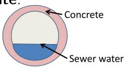
**At Bottom**: After a while, sludge is piled up and becomes anaerobic.
