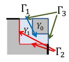
Assumption 5. On  $\Gamma_1$  H<sub>2</sub>SO<sub>4</sub>(aq) and CaCO<sub>3</sub> react and produce Gypsum.  $\eta$ : rate of this reaction  $w_4$ : Concentration of Gypsum
