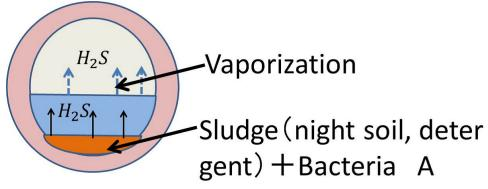
Bacteria A: sulfate reducing bacteria  $SO_4^{-2} + 2C + H_2O \rightarrow H_2S(aq) + 2HCO_3^ H_2S(aq) \rightleftharpoons H_2S(g)$   $H_2S$  (hydrogen sulfide)
