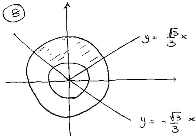
$$y_G = \frac{\int_D y \, dx \, dy}{\int_D dx \, dy} = \frac{\int_{\pi/6}^{5\pi/6} \int_1^2 p \sin \theta \, p \, dp \, d\theta}{\int_{\pi/6}^{5\pi/6} \int_1^2 p \, dp \, d\theta}$$
