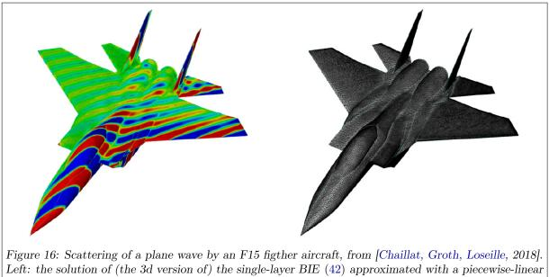
collocation-BEM. Right: the mesh used, with more than 160 000 triangles.
