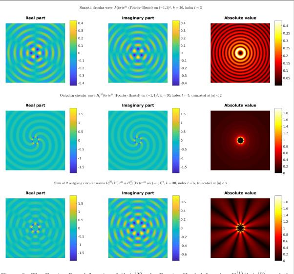
Figure 5: The Fourier-Bessel function  $J_3(kr)e^{i3\theta}$ , the Fourier-Hankel function  $H_5^{(1)}(kr)e^{i5\theta}$ , and the sum of two Fourier-Hankel functions with opposite indices  $H_5^{(1)}(kr)e^{i5\theta} + H_{-5}^{(1)}(kr)e^{-i5\theta}$ . Since the Hankel functions are unbounded at the origin, the field has been truncated to zero in the region where its absolute value is larger than 2.
