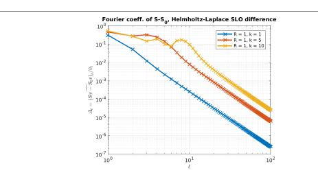
Figure 19: A log-log plot of the Fourier coefficients  $K_{\ell}$  for the operator  $S - S_0$ , difference between Helmholtz and Laplace single-layer operators, on a circle. The coefficients decay as  $K_{\ell} \sim \ell^{-3}$ , so the operator appears to be continuous  $H^s(\partial B_R) \to H^{s+3}(\partial B_R)$ . In particular it is compact  $H^{-\frac{1}{2}}(\partial B_R) \to H^{\frac{1}{2}}(\partial B_R)$ . Compare with the coefficients of S in Figure 15.
