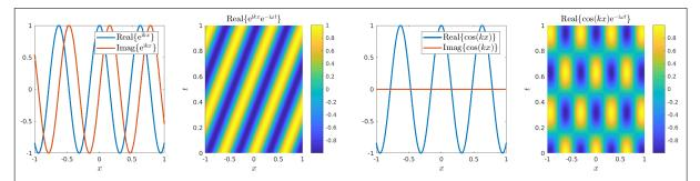
Figure 1: Panel 1: the real and the imaginary part of the one-dimensional propagative wave  $u(x) = e^{ikx}$  over the interval (-1, 1), with k = 10.
