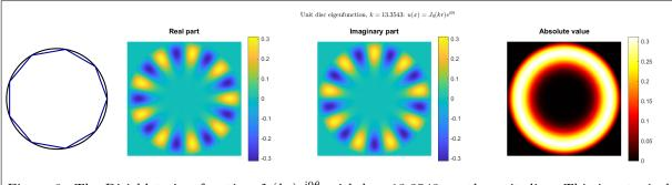
Figure 8: The Dirichlet eigenfunction  $J_9(kr)e^{i\theta\theta}$  with k = 13.3543 on the unit disc. This is a typical "creeping wave" or "whispering gallery mode", as it is concentrated along the boundary of the domain.
