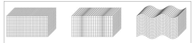
Figure 3: The deformation of an elastic medium perturbed by plane waves. Left: the unperturbed medium. Centre: a longitudinal plane wave  $de^{ik\mathbf{x}\cdot\mathbf{d}}$ . Right: a transverse plane wave  $Ae^{ik\mathbf{x}\cdot\mathbf{d}}$  with  $\mathbf{A}\cdot\mathbf{d}=0$ . In this example the wave propagates horizontally ( $\mathbf{d}=(1,0,0)$ ) and  $\mathbf{A}=(0,0,1)$ . See §1.4 and Exercise 2.3. Acoustic waves are longitudinal waves, since fluids cannot support transverse waves.
